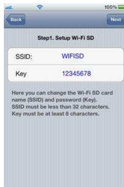
Step 1. Modify the Wi-Fi SD SSID and Key or tap Next to skip this step
